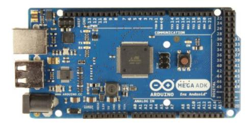
The Arduino ADK is a microcontroller board based on the ATmega2560 . It has a USB host interface to connect with Android based phones, based on the MAX3421e IC. It has 54 digital input/output pins (of which 14 can be used as PWM outputs), 16 analog inputs, 4 UARTs (hardware serial ports), a 16 MHz crystal oscillator, a USB connection, a power jack, an ICSP header, and a reset button. Following is the link for its datasheet, if someone want to refer it in case
