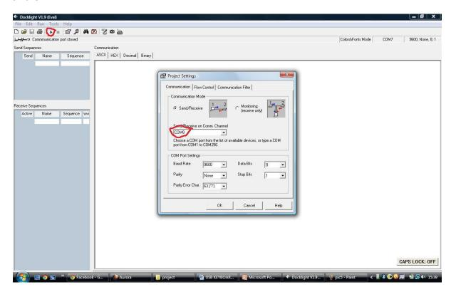
Enter the port at which drivers are installed and press play button to run the communication between Bluetooth module and docklight
