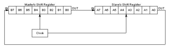
The data is transferred one bit at a time between the master and the slave, and at the end of 8 cycles the data is completely exchanged.
