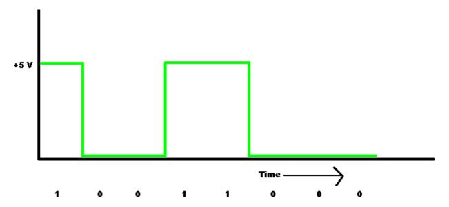
Now as it might be clear there should be some way to tell this signal from 1010 of 100010 of some other. For this, we can do either of two things, set a standard that at a particular rate, the data will be transferred and we keep checking for voltage at time moments T, 2T, 3T so on, or we also send a clock pulse at the same time. Like we decide that whenever we send a new signal, we will make the clock 1. Then the clock signal would look like:
