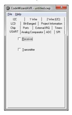
As you can see, you can set the USART to either receive, transmit, or both. Checking the appropriate checkboxes will enable more options for configuration.
