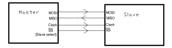
MOSI is **M**aster **O**ut **S**lave **I**n, so it is the channel where the master sends the data to the slave and the slave receives it.
