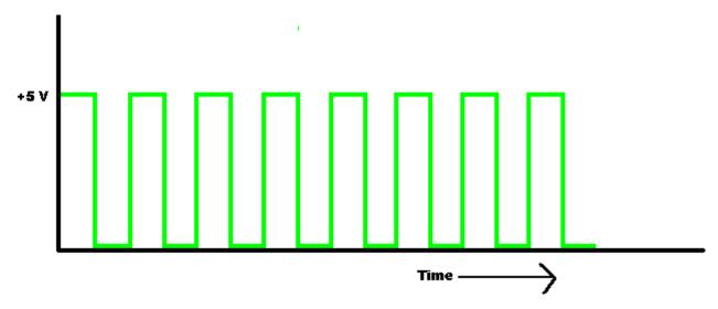
Now if the receiving machine reads the incoming data at negative edges, it will always read what the sender actually meant. This the concept of synchronous data transfers. The sender and the receiver are synchronized by a clock pulse.
