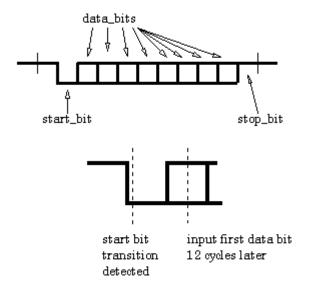
When the entire data word has been sent, the transmitter may add a Parity Bit that the transmitter generates. The Parity Bit may be used by the receiver to perform simple error checking. Then at least one Stop Bit is sent by the transmitter.
