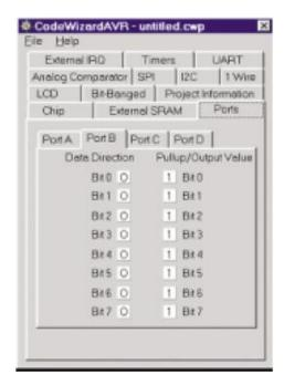
The default setting is to have the ports for all the target systems to be inputs.
