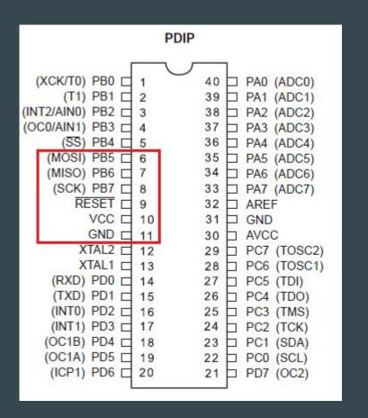
After making connections of programmer, open your windows command prompt and using specific avrdude commands you can upload your program onto AVR chip
