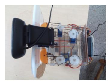
Fig. 1. Top view of eye mechanism.
