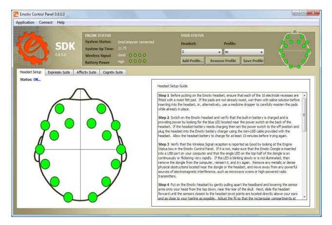
above is the image of the control panel of emotive headset. Green dots here represent the signal received is good.
