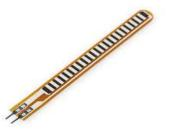
a fixed resistor (not changing) that we can use for that comparison (We are using a 33K resistor). This is called a voltage divider and divides the 5v between the flex sensor and the resistor.
