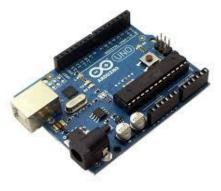
AVR microcontroller with complementary components to facilitate programming and incorporation into other circuits. An important aspect of the Arduino is the standard way that connectors are exposed, allowing the CPU board to be connected to a variety of interchangeable add-on modules known as shields.
